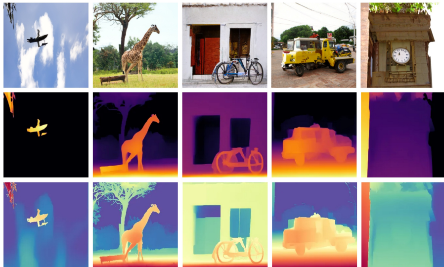
Figure 4: Examples of Depth Estimation Results on NYU Depth V2. The first row illustrates the test images , the second row presents the prediction outcomes from the baseline model (DepthFormer (Li et al. 2022)), and the third row demonstrates the prediction outcomes after incorporating synthetic annotated data generated by FlexDataset during training. FlexDataset enhances the performance of the targeting perception model (DepthFormer).
